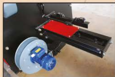
Martinetto idraulico griglia mobile Moving grate hydraulic cylinder
